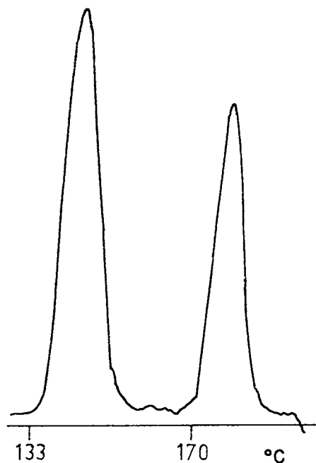
Figure 1 DTA curves of a mixture of dihydrate (50%) and hemihydrate (50%).
